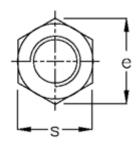
$\begin{array}{lll} d & = M6 \\ d \; max & = 6.75 \\ d \; min & = 6.0 \\ e & = 11.05 \\ m1 \; max = 3.2 \\ m1 \; min & = 2.90 \\ m2 & = 2.3 \end{array}$
